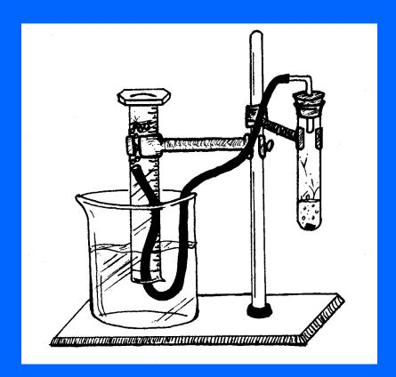
Put the rubber hose inside the cylinder.
