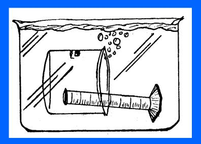
• Submerse a 100 ml cylinder and a 1000 ml beaker in the sink. Make sure that there are no bubbles in the top of the cylinder. Keep the cylinder inverted when they are removed from the water
